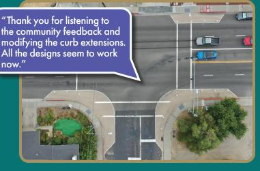
Crosswalk lines were extended over the painted area to align with a new radius created by the repositioned bollards. Bollards at the edges of the extensions were removed for bicyclist safety.
