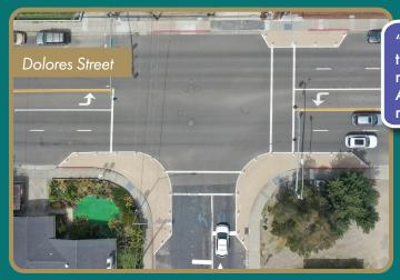
A recessed stop bar was installed at this intersection, along with mirrored curb extensions, for pedestrian safety and to minimize conflicts between the turning LAVTA bus and vehicles idling at the intersection.
