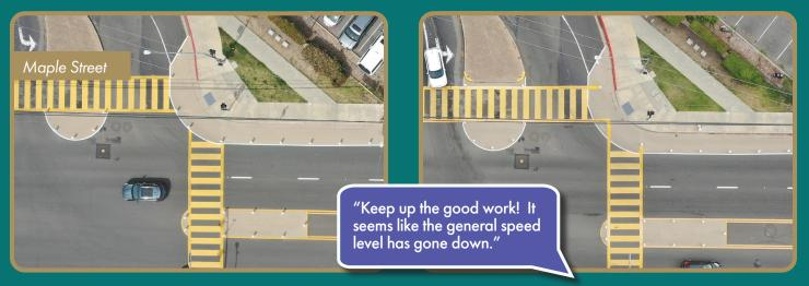
At Maple Street, curb extensions and painted medians reduced crossing distances for students walking to Livermore High School. Bollards were similarly repositioned within the northeast curb extension to ease the right turn of the LAVTA bus at this intersection.
